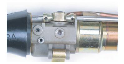
When replacing the Electrical Cable on a Cobra Gold make sure to properly place the connectors back into the handle opening above the potentiometer assembly. Use the picture below as a guide for proper placement.
